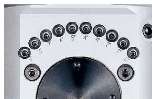
Indexing mechanism in 1° increments
