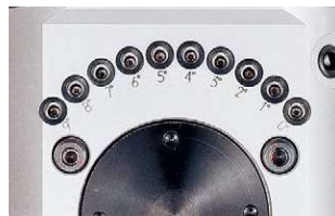
Indexing mechanism in 1° increments
