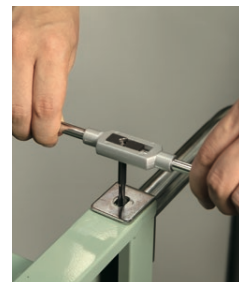
When hand tapping, always use tap wrench
