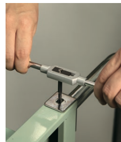
Hand tapping using a tap handle.
