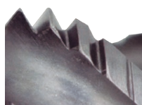
Close-up of VUSP after Tapping of 250 Holes
