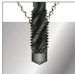
Chips from a tapped hole.
